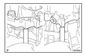
(c) Carefully tap the transmission case with a brass bar and hammer and remove it from the transaxle cace.
