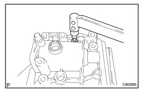
(d) Using a hexagon wrench and torque wrench install the reverse restrict pin plug to the manual transmission case.
