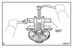
(b) Using SST and a hammer, remove the front differential case rear tapered roller bearing (inner race) from the from differential case.
