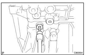
(d) Coat the shift detent ball plug with sealant, install it with using a hexagon wrench.
