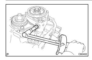
(b) Coat the gear shift lock fork bolt with sealant, install it to the gear shift fork No. 3.
