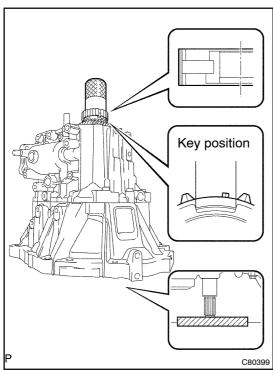
(b) Using SST and a hammer, install the transmission clutch hub No. 3 to the input shaft.
