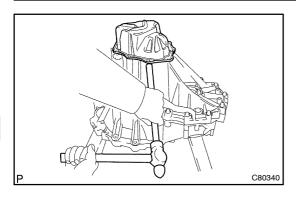
(b) Carefully tap the projection of the manual transmission case cover sub-assy with a brass bar and hammer and remove it.
