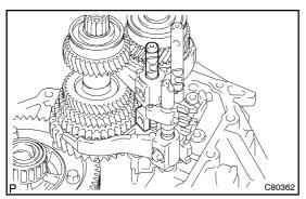
(b) Remove the gear shift fork shaft No. 2 and gear shift head No. 1 from the front transaxle case.
