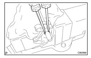
(d) Using 2 screwdrivers and hammer, tap out the snap ring from the shift fork shaft No. 3.
