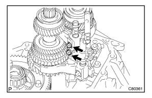
(b) Coat the 2 shift lock bolts with sealant, install it to the gear shift fork No. 2 and shift head No. 1.
