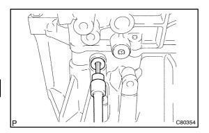
(c) Using a hexagon wrench, remove the shift detent ball plug from the front transaxle case.
