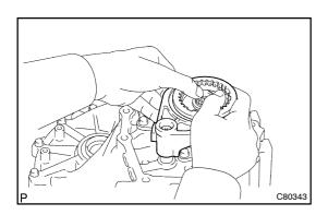
(b) Remove the No. 3 hub sleeve and gear shift fork No. 3 from the transmission clutch hub No. 3.
