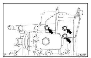
(b) Install the 3 bolts the engine mounting bracket LH to the manual transmission case.
