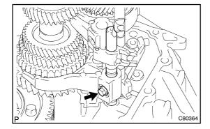
(b) Remove the gear shift fork lock bolt and gear shift fork shaft No. 1 from the gear shift fork No. 1.
