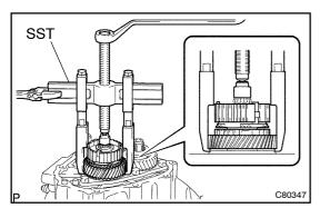
(b) Using SST, remove the transmission clutch hub No. 3, 5th gear and synchronizer ring from the input shaft.
