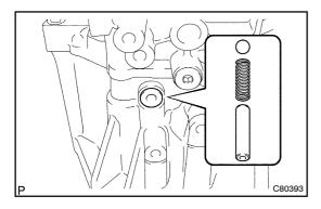
(c) Install the shift detent ball, shift detent ball compression spring and shift detent ball spring seat No.1 to the front transaxle case.
