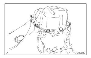
(b) Install the 9 bolts with manual transmission case cover to the manual transmission case.
