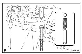
(b) Using a magnetic finger, remove the 2 seats, springs and balls from the manual transmission case.
