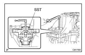
(d) Using SST and a torque wrench, measure the preload.
