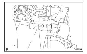
(b) Coat the 2 shift detent ball plugs with sealant, install them with a hexagon wrench.
