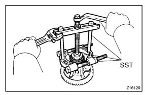
(b) Using SST, remove front differential case front tapered roller bearing (inner race) from the front differential case. SST 09950-00020, 09950-00030, 09950-40011 (09957-04010), 09950-60010 (09951-00360)
