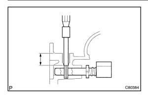
(b) Using a pin punch ( $\phi$  5 mm) and hammer, install the slotted pin to the reverse restrict pin assy.
