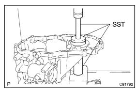
(b) Using SST and a press, front differential case rear tapered roller bearing (outer race) with shim to the transmission case.
