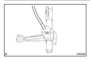
(c) Using a magnetic finger, remove the 2 reverse shift fork balls from the reverse shift fork.
