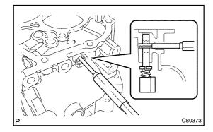
(b) Using a pin punch (φ 5 mm) and hammer, drive out the slotted spring pin and reverse restrict pin assy from the manual transmission case.
