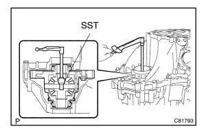
(c) Using SST and a torque wrench, turn the differential case assy right and left 2 or 3 times to allow the bearings to settle.
