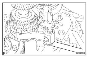
(e) Using a brass bar and hammer, install the shaft snap ring to the gear shift fork shaft No. 1.
