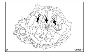
(c) Coat the 3 bolts with sealant, install to the front transaxle case.
