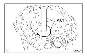
(b) Using SST and a press, install the front differential case front tapered roller bearing (outer race) with shim to the front transaxle case.
