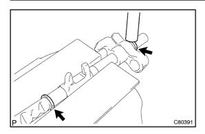
(c) Using a brass bar and hammer, install 2 shift fork shaft snap rings to the shift fork shaft No. 3.
