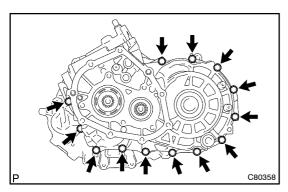
(b) Remove the 13 bolts from the manual transmission case.
