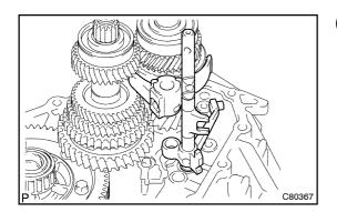
(b) Remove the shift fork shaft No. 3, reverse shift fork and gear shift fork No. 2 from the front transaxle case.
