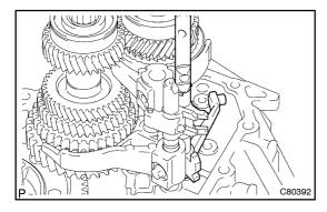
(d) Coat the shift fork shaft No. 3 with gear oil, install it.
