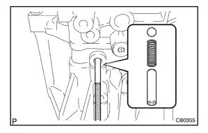
(d) Using a magnetic finger, remove the seat, spring and ball from the front transaxle case.
