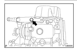
(b) Remove the bolt and selecting bell crank assy from the manual transmission case.
