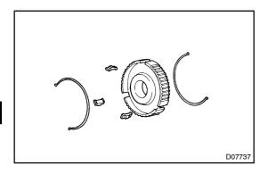
(c) Remove the 3 synchromesh shifting keys and 2 synchromesh shifting key springs from the transmission clutch hub No. 3.
