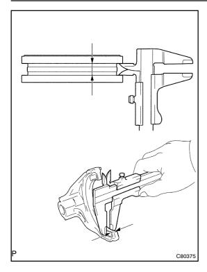
(c) Using a vernier calipers, inspect the transmission hub sleeve No. 3 and gear shift fork No. 3 as shown in the illustration.
