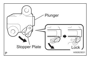
(c) Lower the stopper plate with the plunger pushed to the end, then lock the plunger.
