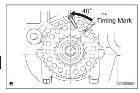
(c) Align the timing marks of the camshaft timing sprocket, camshaft timing gear and crankshaft timing sprocket with each mark plate (colored in yellow) of the timing chain.
