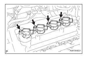
(e) Remove the bolt and ignition coil.
