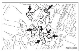
(b) Remove the 3 bolts and 4 nuts, then remove the engine mounting insulator RH.
