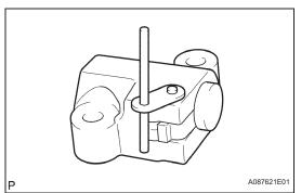
(d) Insert a 3.0 mm (0.118 in.) diameter bar into the hole of the stopper plate with the plunger locked. HINT:
