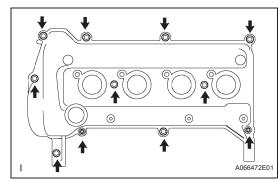
(f) Remove the 9 bolts and 2 nuts, then remove the cylinder head cover.
