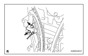
(e) Remove the 2 bolts and chain tensioner.
