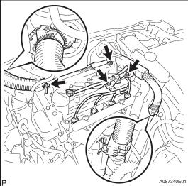
(f) Install the wire harness and brake master cylinder reservoir cover with the 3 bolts.
