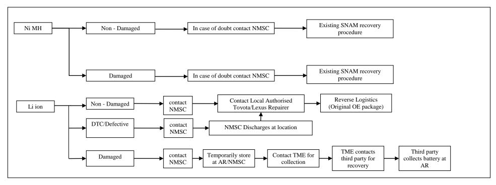
According to the UN regulations for the transport of dangerous goods, Li-Ion batteries can't be shipped to authorized Retailers without a safety diagnosis. Please refer to HV Battery Recovery inspection procedure in TechDoc or to the procedure published in the International Dismantling Information System (IDIS – www.idis2.com).
