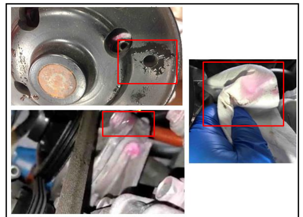
Figure 4. Active Leak Leak – Wet Coolant Residue/Drips (Replace the Water Pump)
