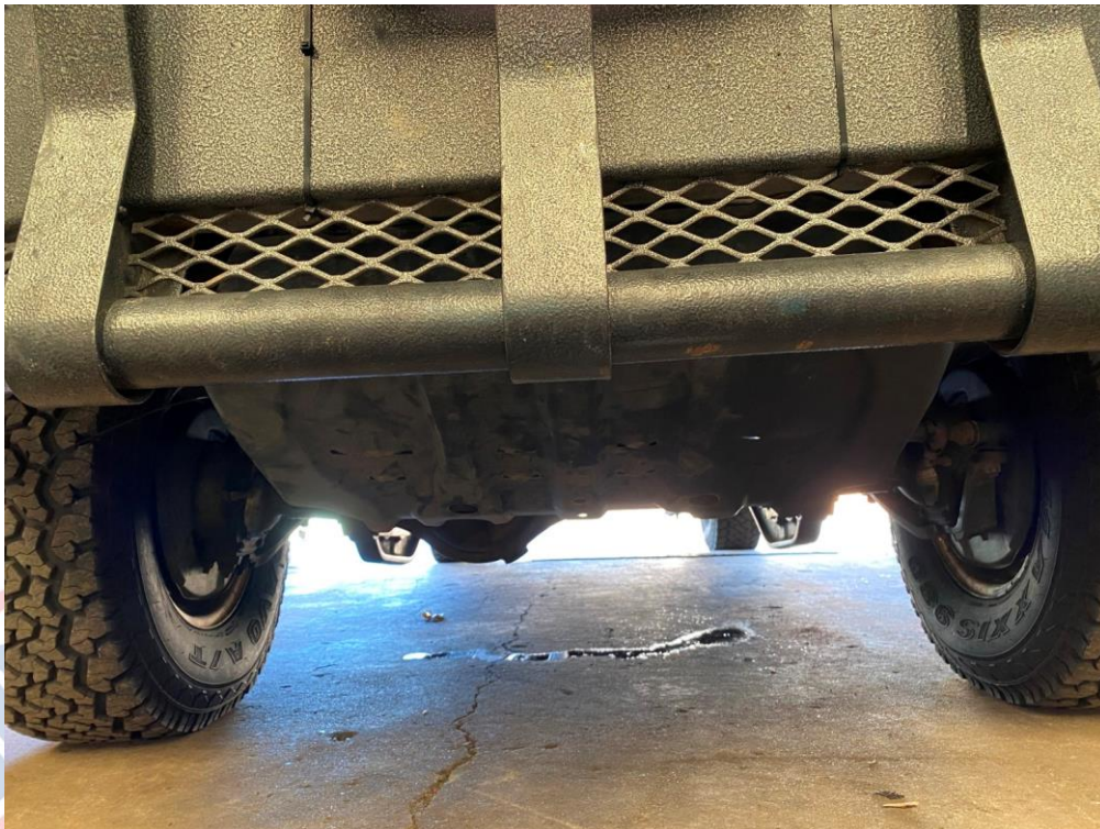
Air dam fitted under front of vehicle to see if would help extract hot air from the engine bay.
