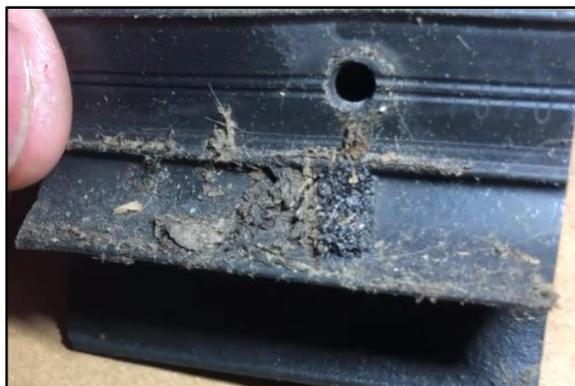
**Figure 5. Example of Debris on Drain Hole**
