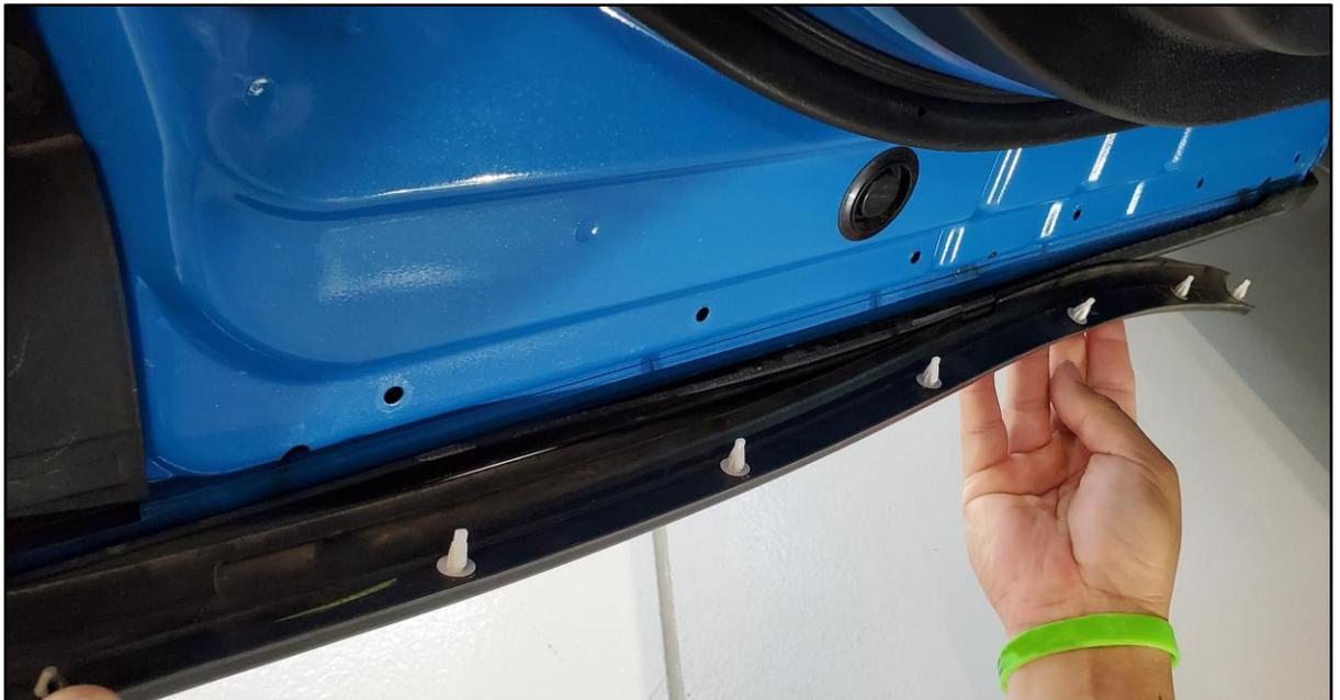
8. Ensure the cut window on the weatherstrip molding and the drain hole align properly.
