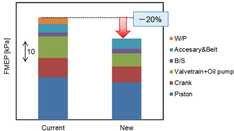
**Figure 34:** FMEP comparison (2000rpm motoring)
