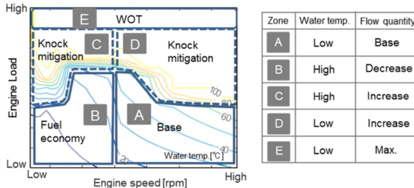
**Figure 22:** Strategy of water flow and temperature control
