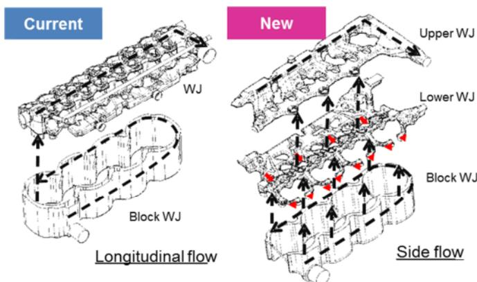
**Figure 19:** Structure of water jackets
