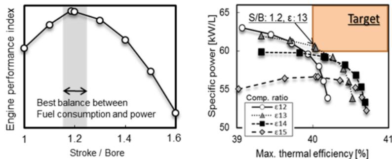
**Figure 7:** Effect of S/B ratio on engine performance and relationship between maximum thermal efficiency and specific power
