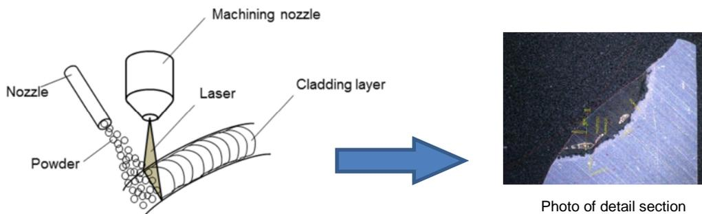
**Figure 10:** Laser cladded valve seat
