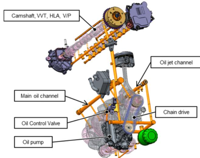
**Figure 26:** Lubrication system
