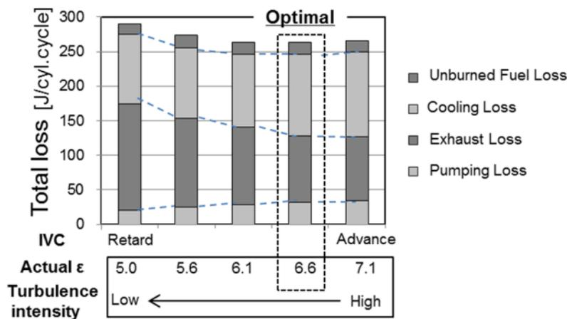
**Figure 18:** Sensitivity of various losses according to IVC
