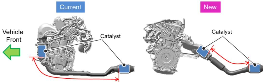
**Figure 29:** Exhaust layout on vehicle
