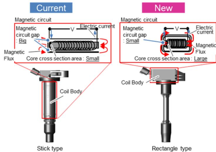
Figure 14: Comparison of current and new ignition coil
