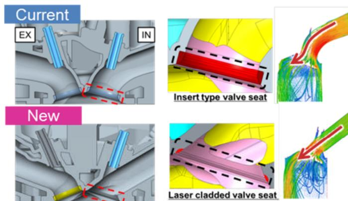
**Figure11:** Comparison of intake port
