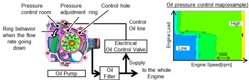
**Figure 25:** Electric control-type variable capacity oil pump
