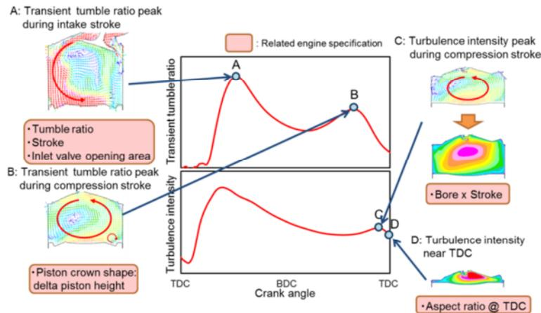
**Figure 8:** In-cylinder flow characteristic and related engine specification
