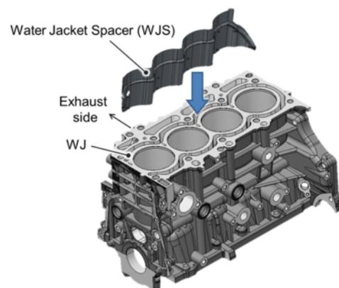
**Figure 20:** Water jacket spacer
