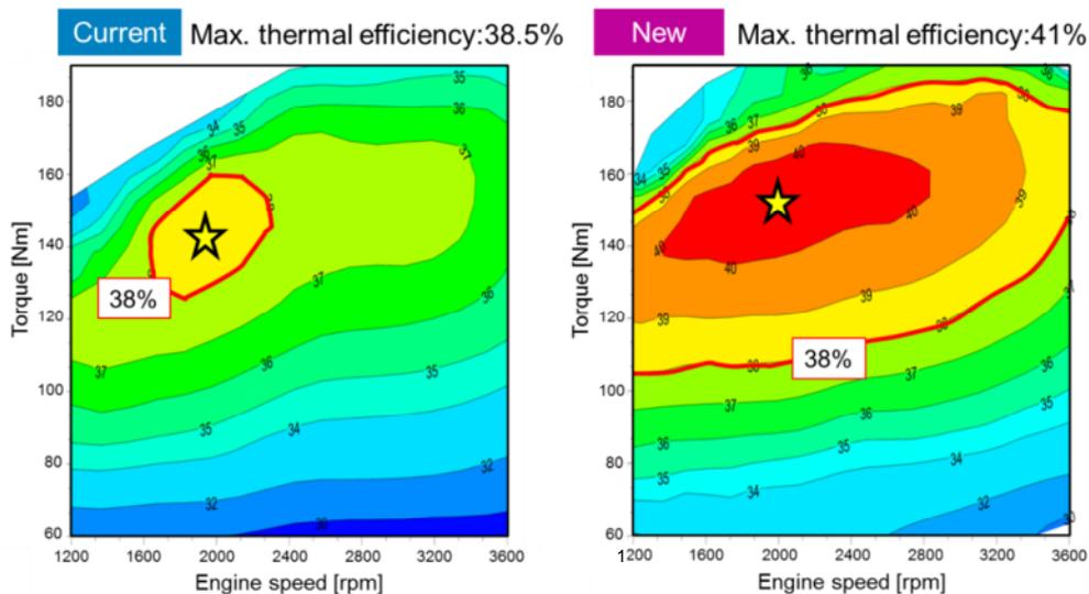
**Figure 40:** Comparison of thermal efficiency map (HV)
