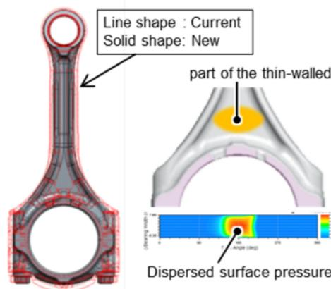
**Figure 16:** Optimized connecting rod
