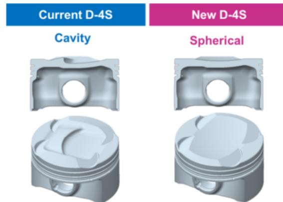
**Figure 12:** Comparison of current and new D-4S piston crown shape
