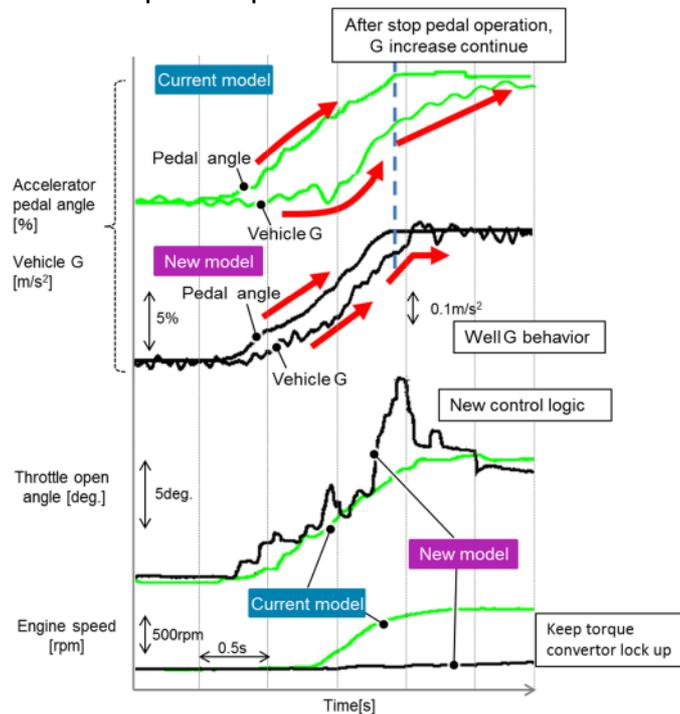
**Figure 45:** Comparison of G controllability under sweep acceleration (50 km/h, accelerator pedal angle: 10 to 20% /1 sec).
