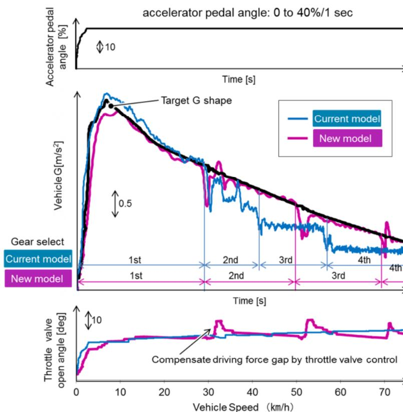
**Figure 44:** Comparison of vehicle G behavior under sweep acceleration
