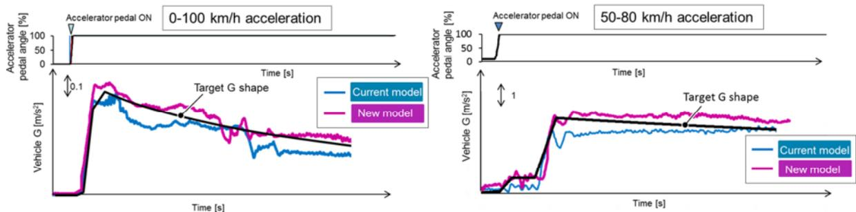
Figure 43: Target G waveform under WOT acceleration
