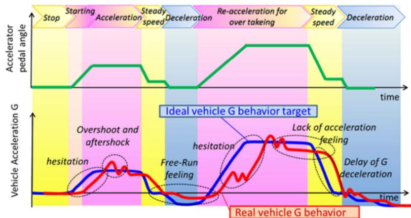
**Figure 41:** Target dynamic performance concept for TNGA powertrain.
