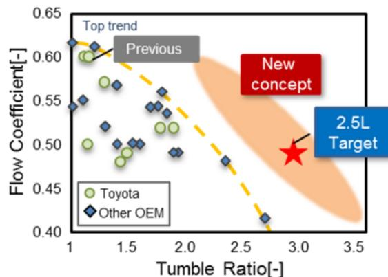
**Figure 9:** Target of intake port performance
