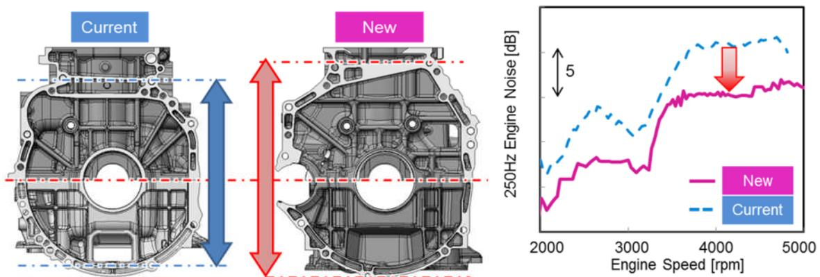
**Figure 35:** Comparison of engine contact surface shape and 250Hz engine noise
