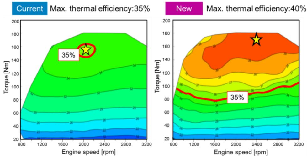
**Figure 39:** Comparison of thermal efficiency map (conventional vehicle)
