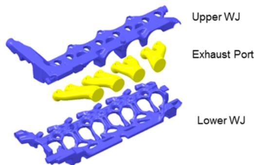
Figure 27: Exhaust port and water jackets structure
