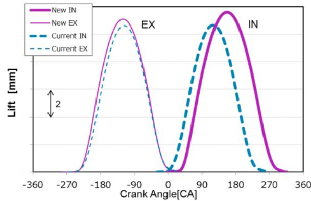
**Figure 17:** Comparison of valve timing
