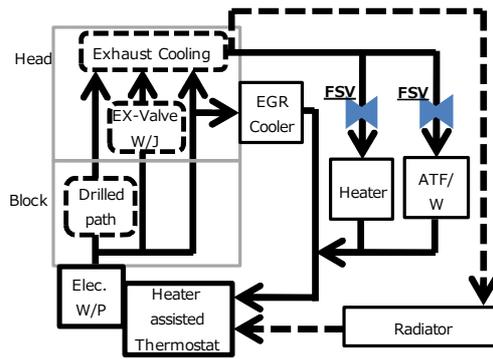
**Figure 23:** Cooling system circuit (for conventional engine)
