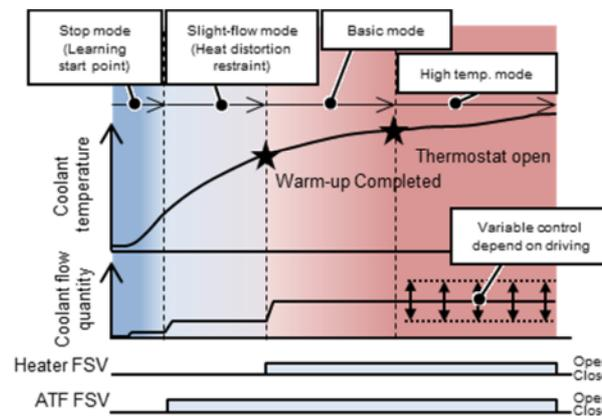
**Figure 24:** Example of control with FSV and coolant flow quantity in warm-up process
