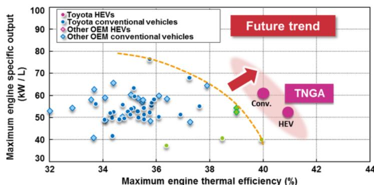
**Figure 3:** Trend and targets of specific power and thermal efficiency
