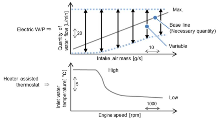
**Figure 21:** Control of electric water pump and heater assisted thermostat
