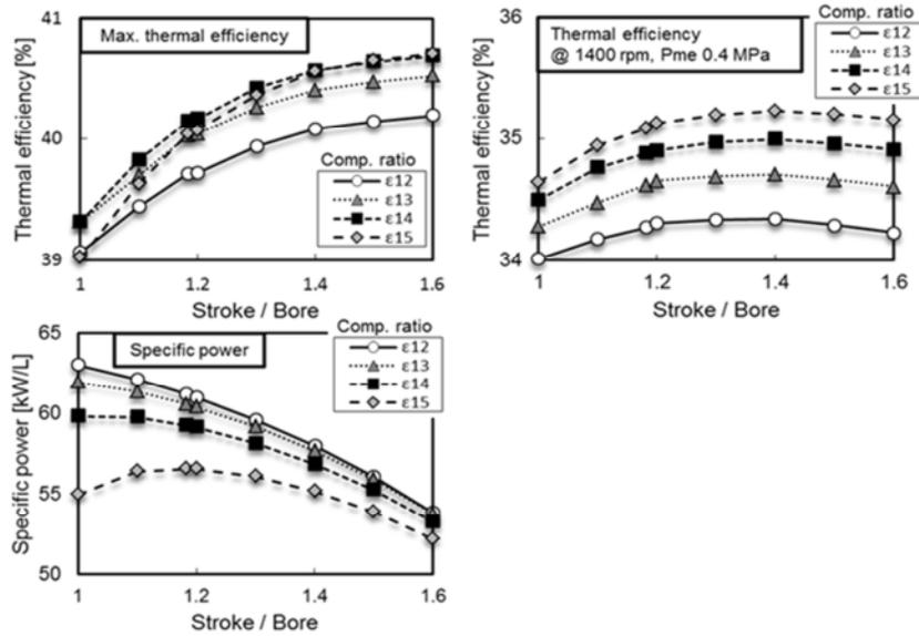
**Figure 6:** Effect of S/B ratio on engine performance
