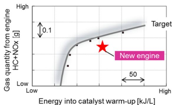
**Figure 31:** Target for necessary energy to catalyst in warm-up process
