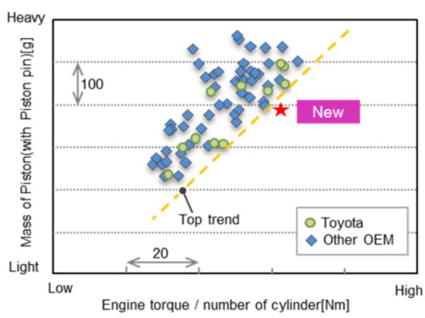
Figure 15: Relationship between piston mass and engine torque per cylinder of NA engines
