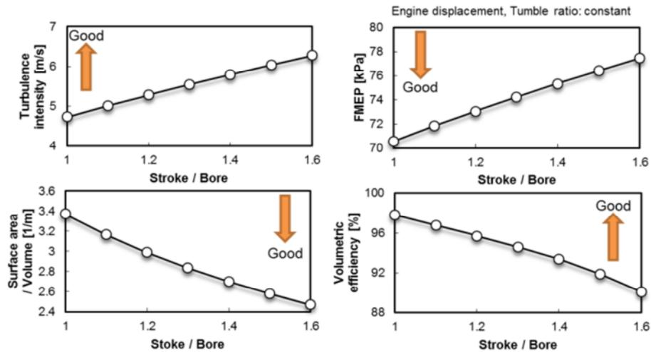
**Figure 5:** Effect of S/B ratio on combustion characteristics
