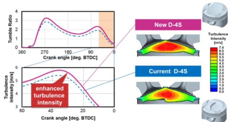
**Figure 13:** Comparison of turbulence intensity between current and new D-4S piston
