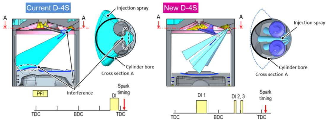
**Figure 33:** Comparison of injection timing and number in catalyst warm-up process
