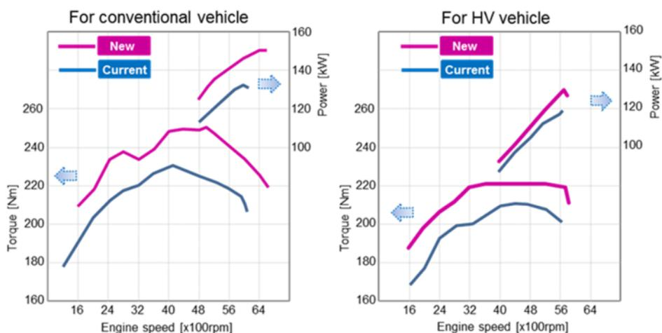
**Figure 38:** The engine power and torque curve
