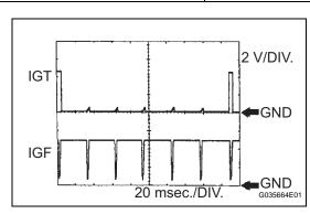
Reference: Inspection using an oscilloscope.
