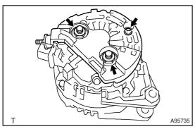
(b) Using a 15 mm socket wrench, remove the screw and 2 nuts, then detach the generator rear end cover.
