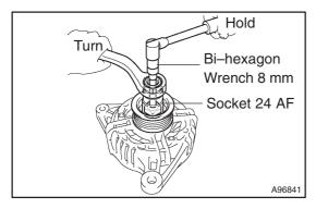
(b) Using a socket 24 AF and a bi-hexagon wrench 8 mm, install the pulley with the spring washer and nut.
