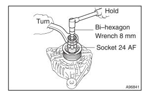
(b) Using a socket 24 AF and bi-hexagon wrench 8 mm, remove the nut and spring washer, then detach the pulley.
