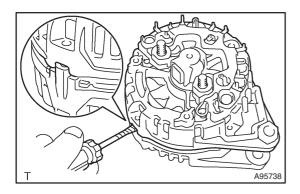
(b) Using a screwdriver, pry out the stator generator with rectifier.
