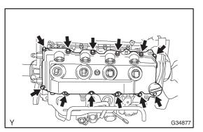
(c) Install the gasket and cylinder head cover with the 10 bolts and 2 nuts.
