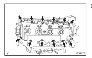
(b) Remove the 10 bolts, 2 nuts, cylinder head cover and gasket.
