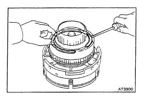
(d) Using a screwdriver, install the snap ring. HINT: Be sure the end gap of the snap ring is not aligned with the cutout portion of the front clutch drum.
