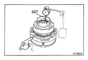
(d) Using SST and a dial indicator, measure the piston stroke by applying and releasing the compressed air (4 - 8 kg/cm2, 57 - 114 psi or 392 - 785 kPa) as shown.
