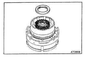
(c) Remove the spring seat and twenty-two return springs.
