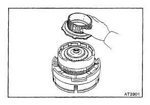
(b) Remove the rear clutch hub.
