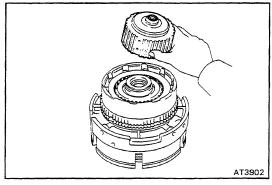
(c) Remove the front clutch hub.
