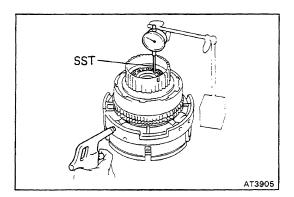
(d) Using SST and a dial indicator, measure the piston stroke by applying and releasing the compressed air
