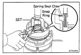
(b) Place SST on the spring seat, and compress the return springs with a shop press.
