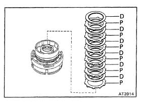
(b) install the six plates and six discs in order:
