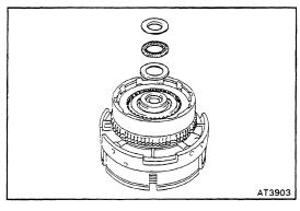
(d) Remove the two races and thrust bearing.
