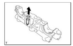
(a) Remove the oil control valve filter .
