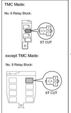
(b) Remove the ST CUT relay from the No. 8 relay block (except TMC made).
