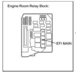
(a) Remove the EFI MAIN fuse from the engine room relay block.
