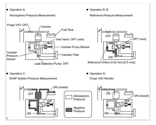
P2420: Vent valve stuck open (vent)
