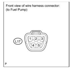
(a) Disconnect the fuel pump connector.
