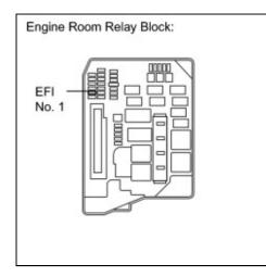
(a) Remove the EFI No. 1 fuse from the engine room relay block.
