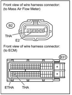
(a) Disconnect the mass air flow meter connector.
