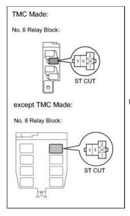
(b) Remove the ST CUT relay from the No. 8 relay block (except TMC made).
