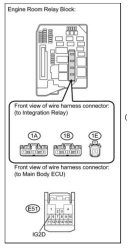
(a) Remove the integration relay from the engine room relay block.
