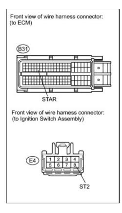
(b) Disconnect the ignition switch assembly connector.
