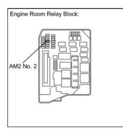
(a) Remove the AM2 No. 2 fuse from the engine room relay block.
