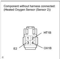
(a) Disconnect the heated oxygen sensor connector.
