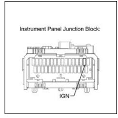
(a) Remove the IGN fuse from the instrument junction block.
