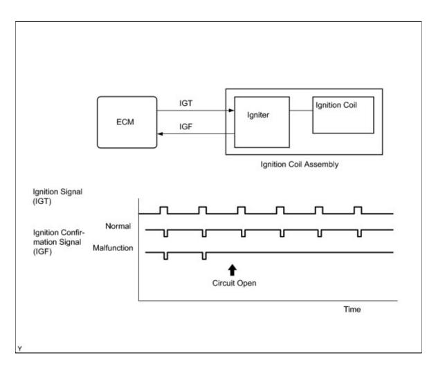
If the ECM does not receive any IGF signals despite transmitting the IGT signal, it interprets this as a fault in the igniter and sets a DTC.
