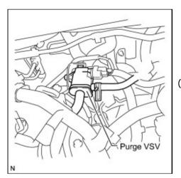
(a) Disconnect the connector and the hoses from the purge VSV.
