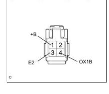
Component without harness connected: (Heated Oxygen Sensor (Sensor 2))
