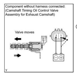
(c) Apply the positive battery voltage to terminal 1 and negative battery voltage to terminal 2. Check the valve operation.
