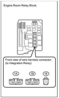
(c) Remove the integration relay from the engine room relay block.
