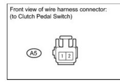
(a) Disconnect the clutch pedal switch connector.
