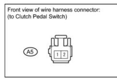
(b) Disconnect the clutch pedal switch connector.
