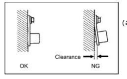
(a) Check the camshaft position sensor (for intake camshaft) installation.
