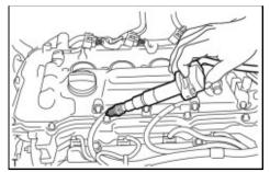
(a) Change the installed spark plug to a known good spark plug.
