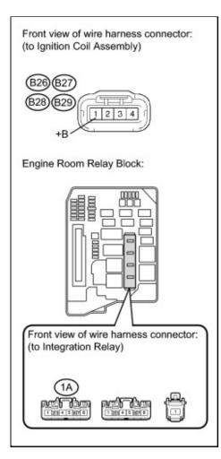
(a) Disconnect the ignition coil assembly connectors.
