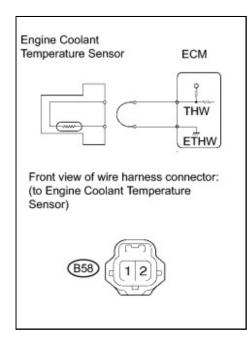
(a) Disconnect the engine coolant temperature sensor connector.
