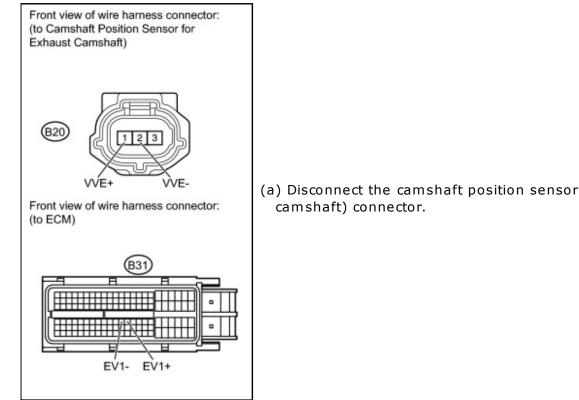
(a) Disconnect the camshaft position sensor (for exhaust
