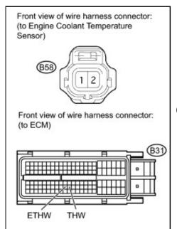
(a) Disconnect the engine coolant temperature sensor connector.
