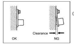
(a) Check the camshaft position sensor (for exhaust camshaft) installation.
