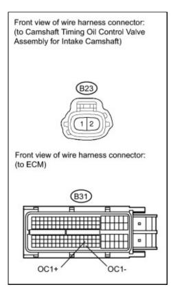
(a) Disconnect the camshaft timing oil control valve assembly (for intake camshaft) connector.
