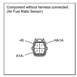
(a) Disconnect the air fuel ratio sensor connector.
