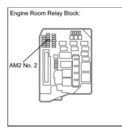
(a) Remove the AM2 No. 2 fuse from the engine room relay block.
