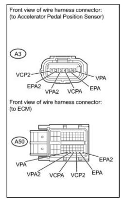
(a) Disconnect the accelerator pedal position sensor connector.
