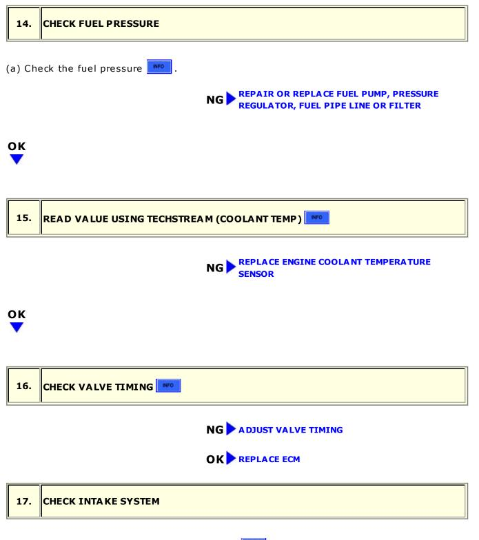
(a) Check the intake system for vacuum leaks .
