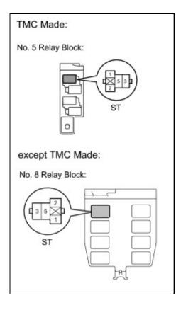
(c) Remove the ST relay from the No. 8 relay block (except TMC made).
