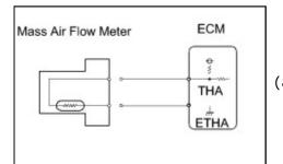
(a) Disconnect the mass air flow meter connector.
