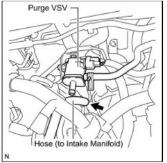
(a) Disconnect the hose (connected to the intake manifold) from the purge VSV.
