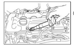
(a) Disconnect the injector connectors to prevent the engine from starting.
