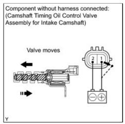
(c) Apply battery voltage to terminals of the camshaft timing oil control valve assembly (for intake camshaft). Check the valve operation.
