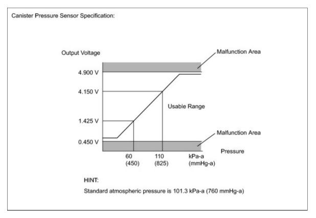
1. DTC P0451: Canister pressure sensor noise or fixed/flat
