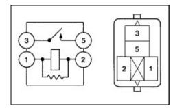
(b) Remove the ST CUT relay from the No. 8 relay block (except TMC made).
