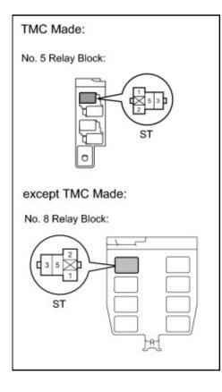
(b) Remove the ST relay from the No. 8 relay block (except TMC made).
