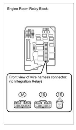
(a) Remove the integration relay from the engine room relay block.
