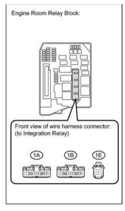
(a) Remove the integration relay from the engine room relay block.
