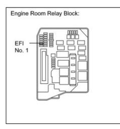
(a) Remove the EFI No.1 fuse from the engine room relay block.
