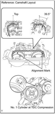
There are no marks on the cylinder head to match-up for the purpose of checking valve timing. Valve timing can only be inspected by lining up the colored plates on the timing chain with the marks on the pulleys. It may be necessary to remove and reinstall the chain to match-up the alignment marks
