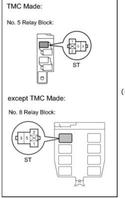
(b) Remove the ST relay from the No. 8 relay block (except TMC made).
