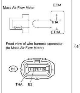
(a) Disconnect the mass air flow meter connector.
