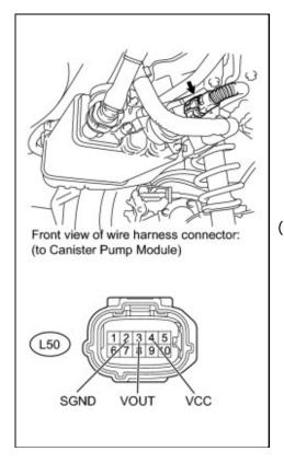
(a) Disconnect the canister pump module connector.
