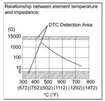
During normal air fuel ratio feedback control, there are small variations in the exhaust gas oxygen concentration. In order to continuously monitor the slight variation of the heated oxygen sensor signal while the engine is running, the impedance\* of the sensor is measured by the ECM. The ECM determines that there is a malfunction in the sensor when the measured impedance deviates from the standard range.
