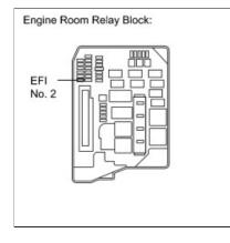
(a) Remove the EFI No. 2 fuse from the engine room relay block.
