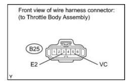
(a) Disconnect the throttle body assembly connector.
