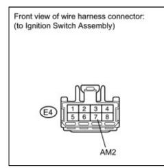
(a) Disconnect the ignition switch assembly connector.
