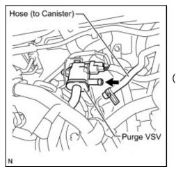
(a) Enter the following menus: Powertrain / Engine and ECT / Active Test / Activate the VSV for EVAP Control.
