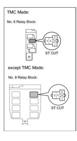
(b) Remove the ST CUT relay from the No. 8 relay block (except TMC made).
