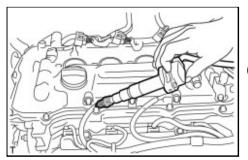
(a) Change the ignition coil assembly to a known good ignition coil.
