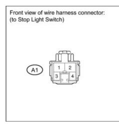
(a) Disconnect the stop light switch connector.
