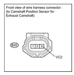
(a) Disconnect the camshaft position sensor (for exhaust camshaft) connector.
