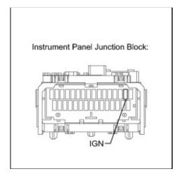
(a) Remove the IGN fuse from the instrument panel junction block.
