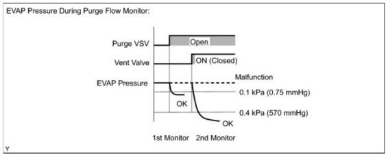
The purge flow monitor consists of two monitors. The 1st monitor is conducted every time and the 2nd monitor is activated if necessary.
