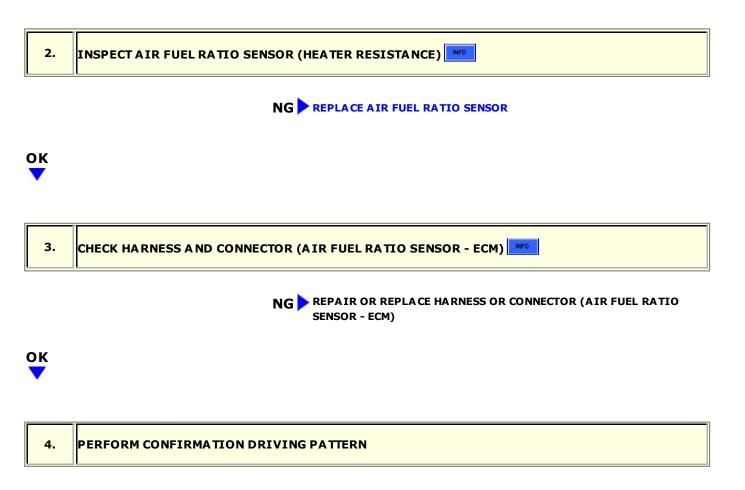
(a) Drive the vehicle referring the Confirmation Driving Pattern.
