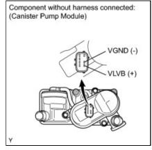
(e) Reconnect the canister pump module connector.
