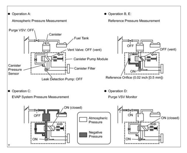
P2420: Vent valve stuck open (vent)
