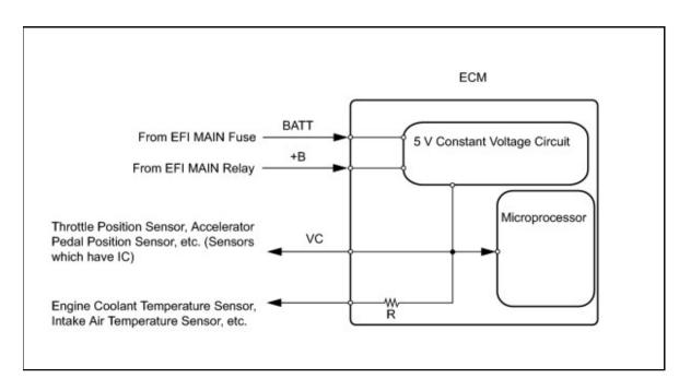
When the VC circuit is short-circuited, the microprocessor in the ECM and sensors that are supplied with power through the VC circuit are inactivated because the power is not supplied from the VC circuit. Under this condition, the system does not start up and the MIL does not illuminate even if the system malfunctions.
