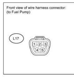
(a) Disconnect the fuel pump connector.
