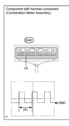
(a) Check the output waveform.
