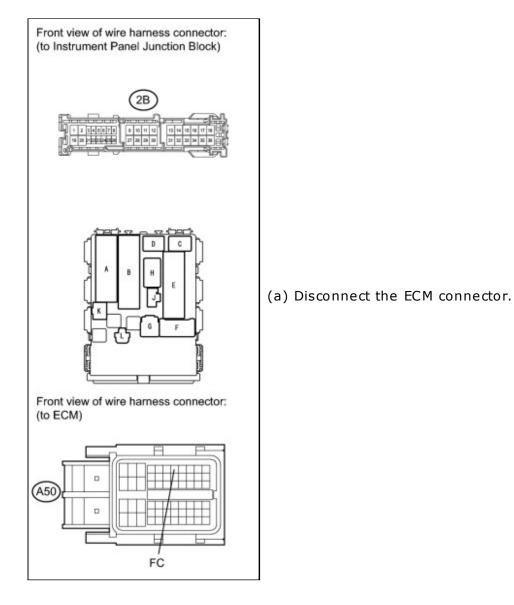
(b) Disconnect the instrument panel junction block connector.
