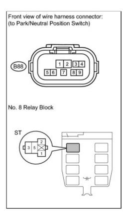
(b) Remove the ST relay from the No. 8 relay block.
