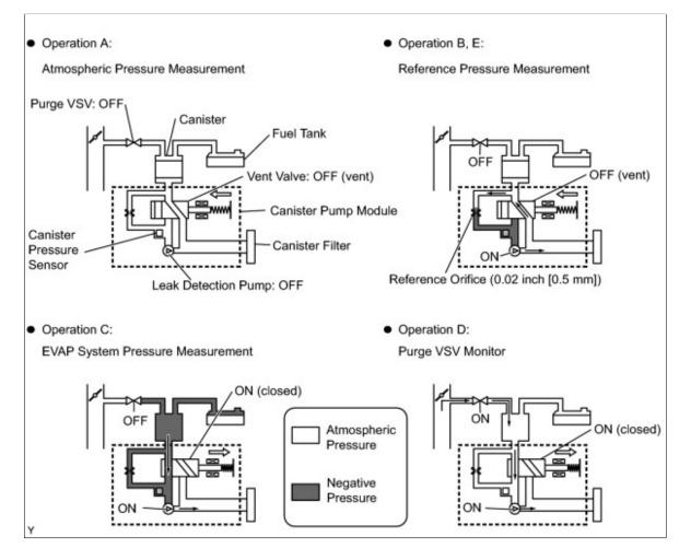
The leak detection pump creates negative pressure through the reference orifice (in operation B and E). When the system is normal, the EVAP pressure is between 724 to 752 mmHg\* and saturated within a minute. If not, the ECM interprets this as a malfunction. The ECM will illuminate the MIL and set DTC if this malfunction is detected in consecutive drive cycles.
