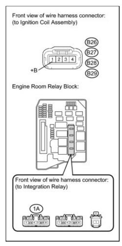
(a) Disconnect the ignition coil assembly connectors.
