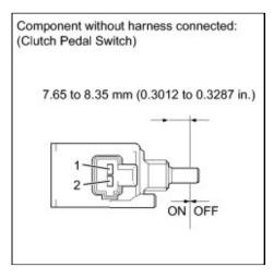
(a) Disconnect the clutch pedal switch connector.
