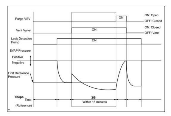
(a) Wait until the EVAP pressure change is less than 0.1 kPa-g (0.75 mmHg-g) for 30 seconds.
