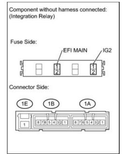
(b) Measure the resistance according to the value(s) in the table below.
